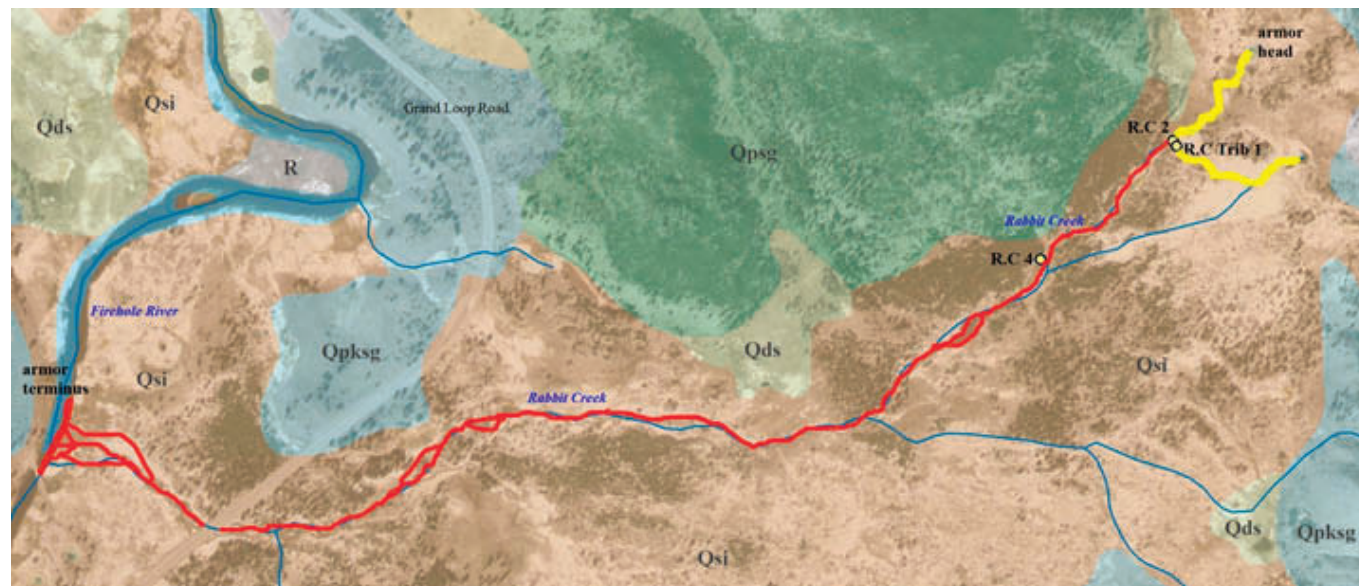
Armored streambed (red) extends the entire length of Rabbit Creek, from near the source of the creek to its confluence with the Firehole River. Near the headwaters (yellow), the armor is blocky rather than continuous.
